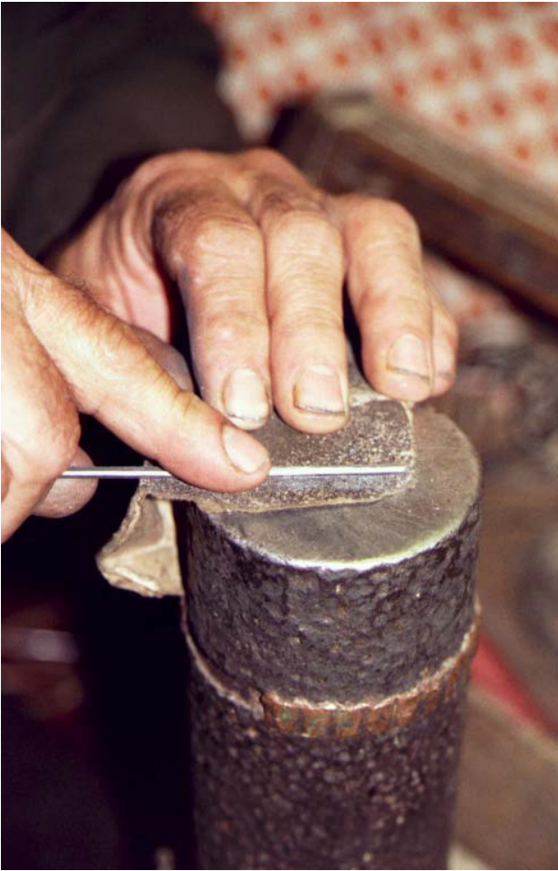
Fig. 7. Shaping the iron rod for the frame.
