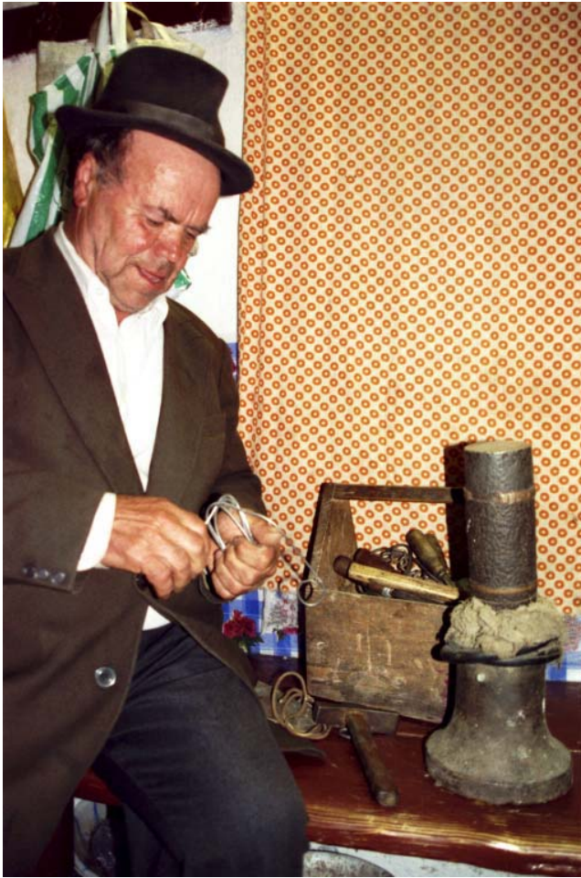
Fig. 5. The first step in drymba-making—Shatruk holds the iron rod that will become the frame.
