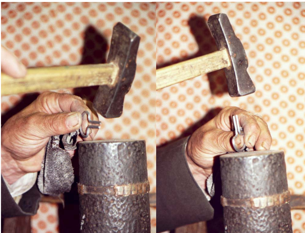
Figs. 9 and 10. Carefully adjusting the frame and arms with some gentle hammer blows.
