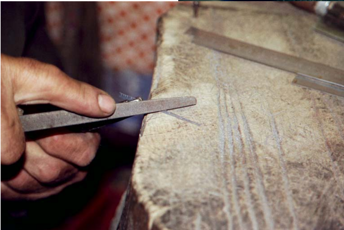
Fig 15, The very precise filing of the tongue (see Fig. 3, top). It is quite impossible to determine the original source of the tongue's material after this operation.
