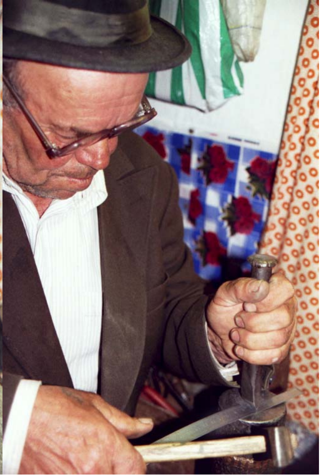
Fig. 13. Cutting the tongue out of Shatruk's multi-use steel ruler.
