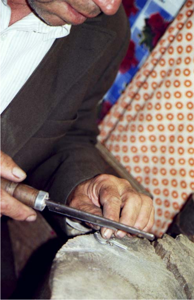
Fig. 11. Sawing the tongue's notch into the frame.
