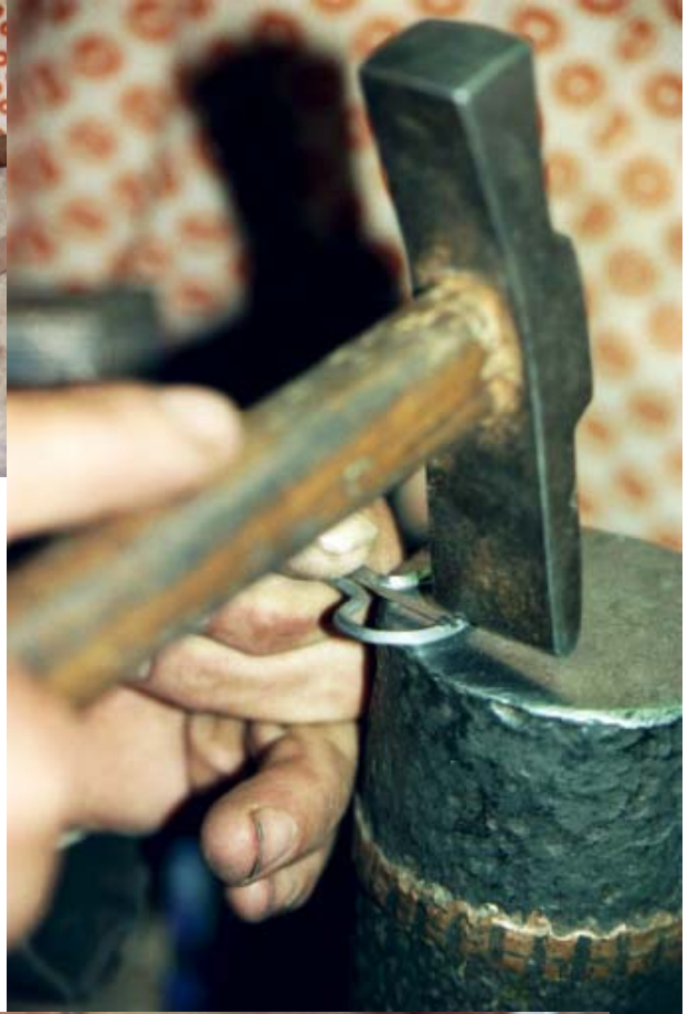
Fig. 14, The tongue requires several operations, from hammering to filing.
